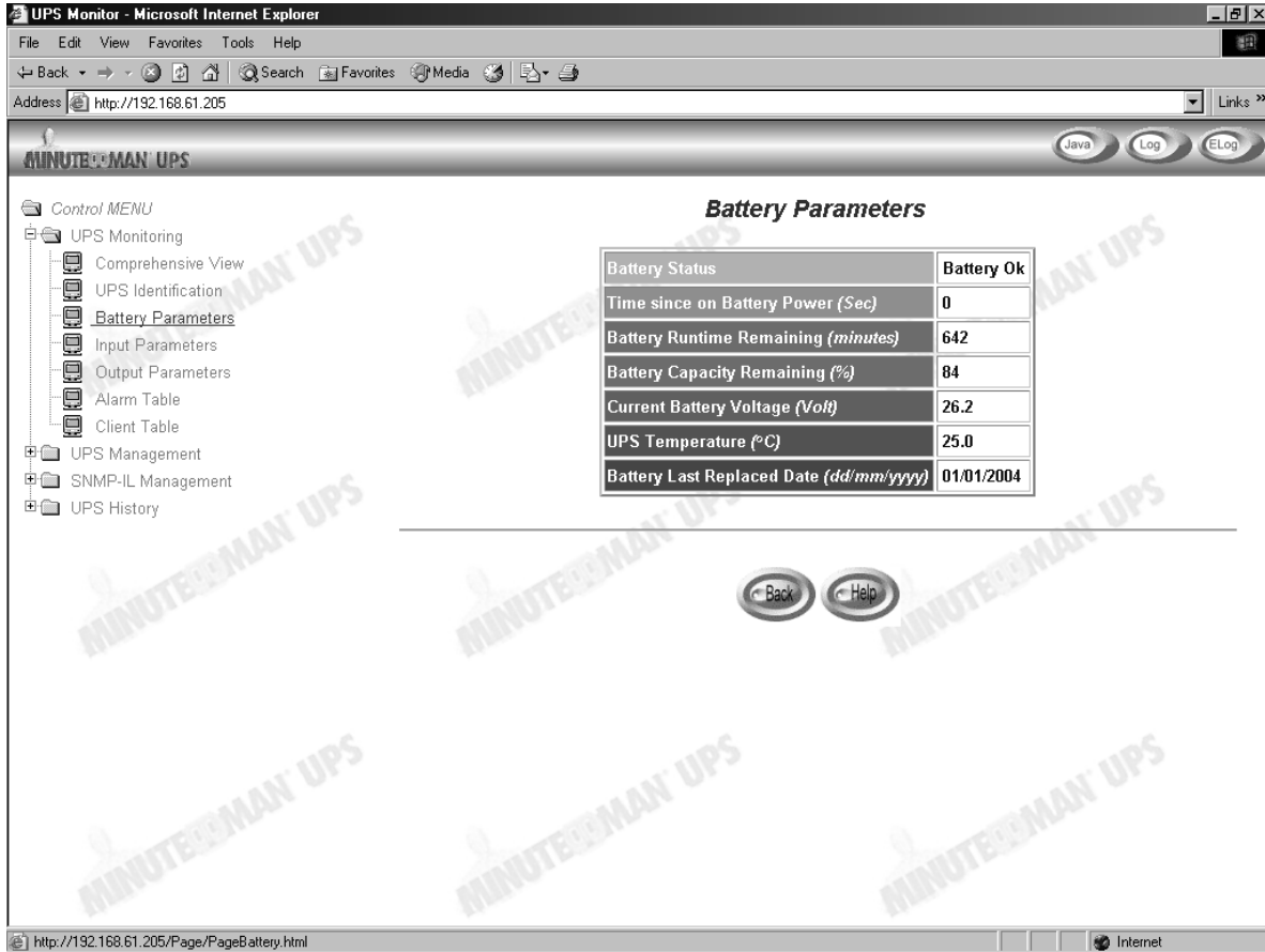
Figure 3-3 SNMP-IL UPS Monitoring page: Battery Parameters.
