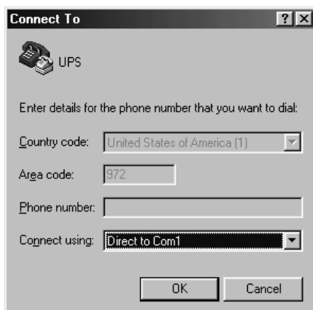
Figure 2-4 Select Direct to COM port connection.
