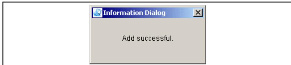
If the deployment is not successful, re-examine the configuration tabs and verify that all 0.0.0.0 IP addresses have been replaced with the correct IP address. Verify other non-default parameters for accuracy. The SIP Application Module and all of its services must be unlocked and enabled. There must be no alarms.
