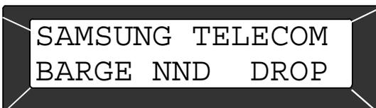
This display shows an investigation of a station that is talking to Samsung Telecom. Investigator can BARGE-in to the conversation, DROP the call from the system or examine further NND information.
